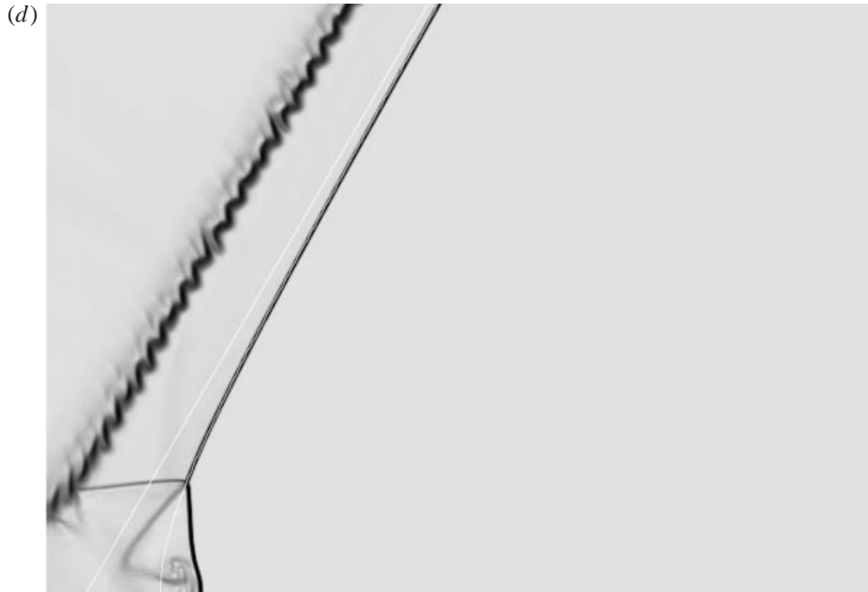
FIGURE 6. Fit of a generalized hyperbola to the computed shock shape for \beta = 20^\circ, 30^\circ, 40^\circ, and 60^\circ . The two straight white lines show the original location of the diaphragm and the asymptote of the hyperbola, which was calculated as the position a plane shock would have reached in the same elapsed time as in the computation of the axisymmetric flow (the latter is missing in the \beta = 30^\circ case). The white curve, which falls almost exactly on the black shock of the computation, is the hyperbola of best fit.
